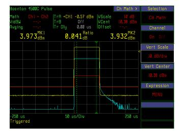
Fig. 4-17b. Markers Indicate Channel 1 power.
