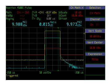
Fig. 4-17c. Markers Indicate Channel 2 power.
